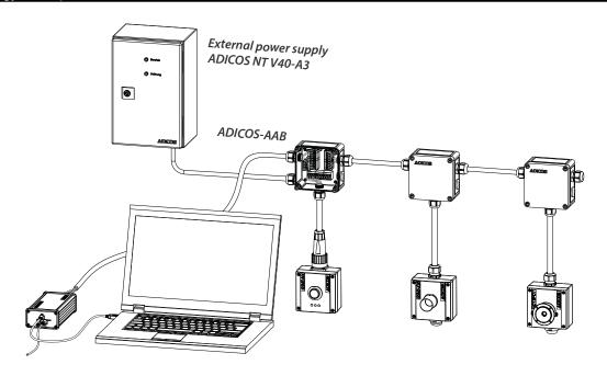
The wiring variants of the ADICOS M-BUSMASTER S differ depending on the system configuration and topology.
