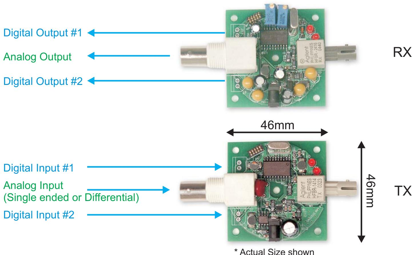
The AFL-200 is a low cost fiber optic link, designed for applications where low cost, high accuracy and low power consumption are essential. The unit can transfer 1 analog signal and 2 digital (TTL) to a distance of more than 1 mile (1.6 Km). The AFL-200 has very low noise and high accuracy.
